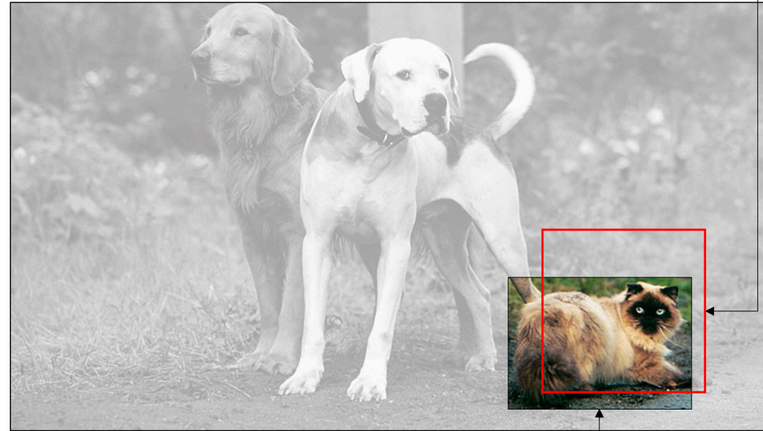
Bounding Box with center-size coordinates (c_x, c_y, w, h)
